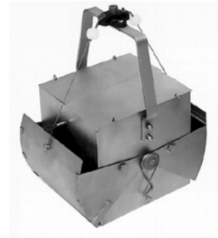
Figure 4: Ekman Sampler Source: NJDEP Field Sampling Procedures Manual (2005)
