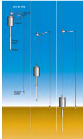
Figure 8 Piston Corer Source: Woods Hole Oceanographic Institution
